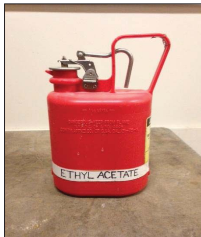
Figure 5.2 – Flammable Safety Can
