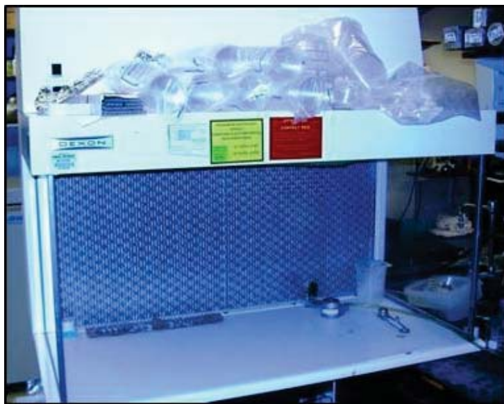
Figure 4.4 – Laminar Flow Clean Bench
