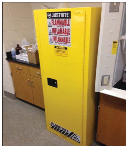
Figure 5.1 – Flammable Storage Cabinet
